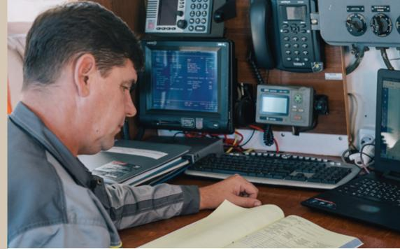
Thuraya SeaStar is a circuit switched voice terminal that meets both corporate and crew calling needs, and can be installed on vessels of all sizes. Offering voice, SMS, narrowband data, and tracking on an intuitive interface, it enables users to make satellite voice calls to normal PSTN phones, mobile phones, and other satellite phones. Thuraya SeaStar can connect to a standard analogue phone and is also ideal as a back-up alternative to VHF and GSM.
